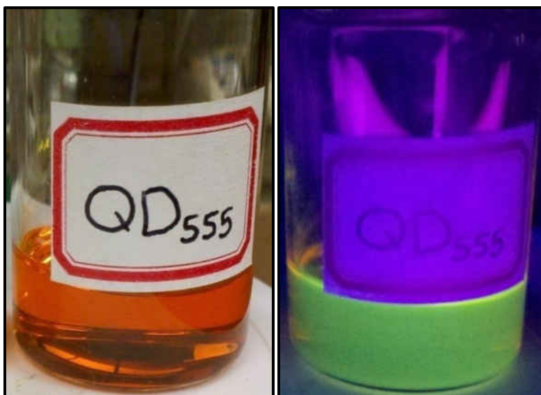
Figure 20. Photos of synthesized red quantum dots with fluorescence emission at 555 nm
