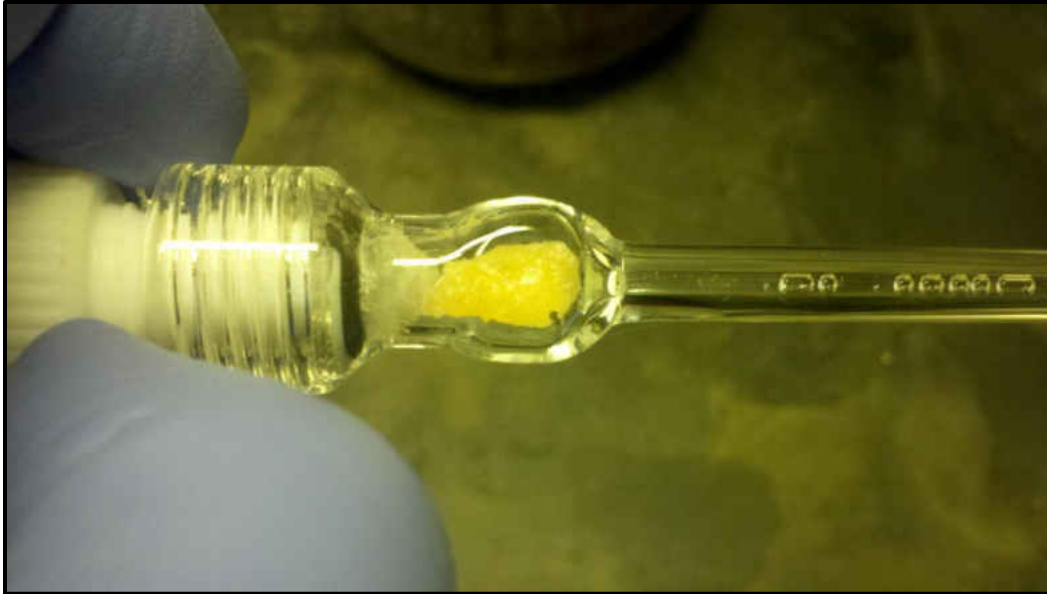
Figure 16. Photo of custom glass flowcell for POCL-FIA with immobilized-quantum dot preparation
