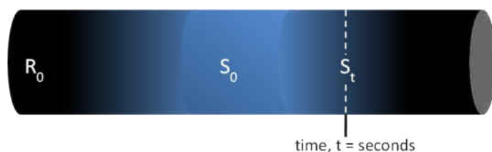
Figure 13. Representation of a dispersed sample gradient within flow injection analyzer.
