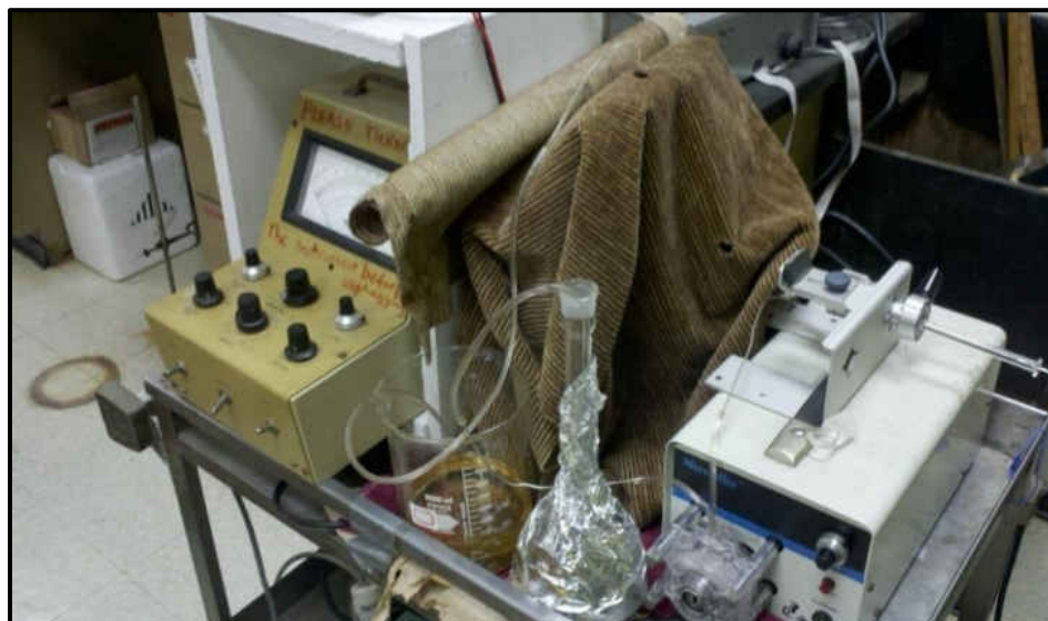
Figure 18. Photo of laboratory built FIA instrument for POCL-FIA measurements with immobilized quantum dots
