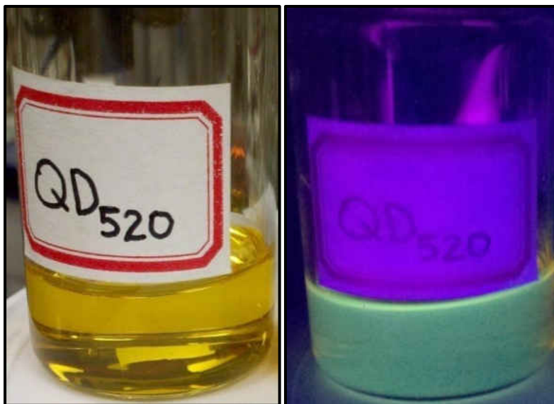
Figure 19. Photos of synthesized yellow quantum dots with fluorescence emission at 520 nm
