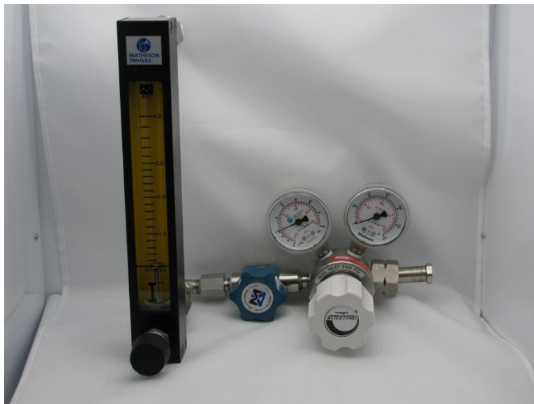
Figure 14 – Gas Regulator and Variable Area Flow Meter
