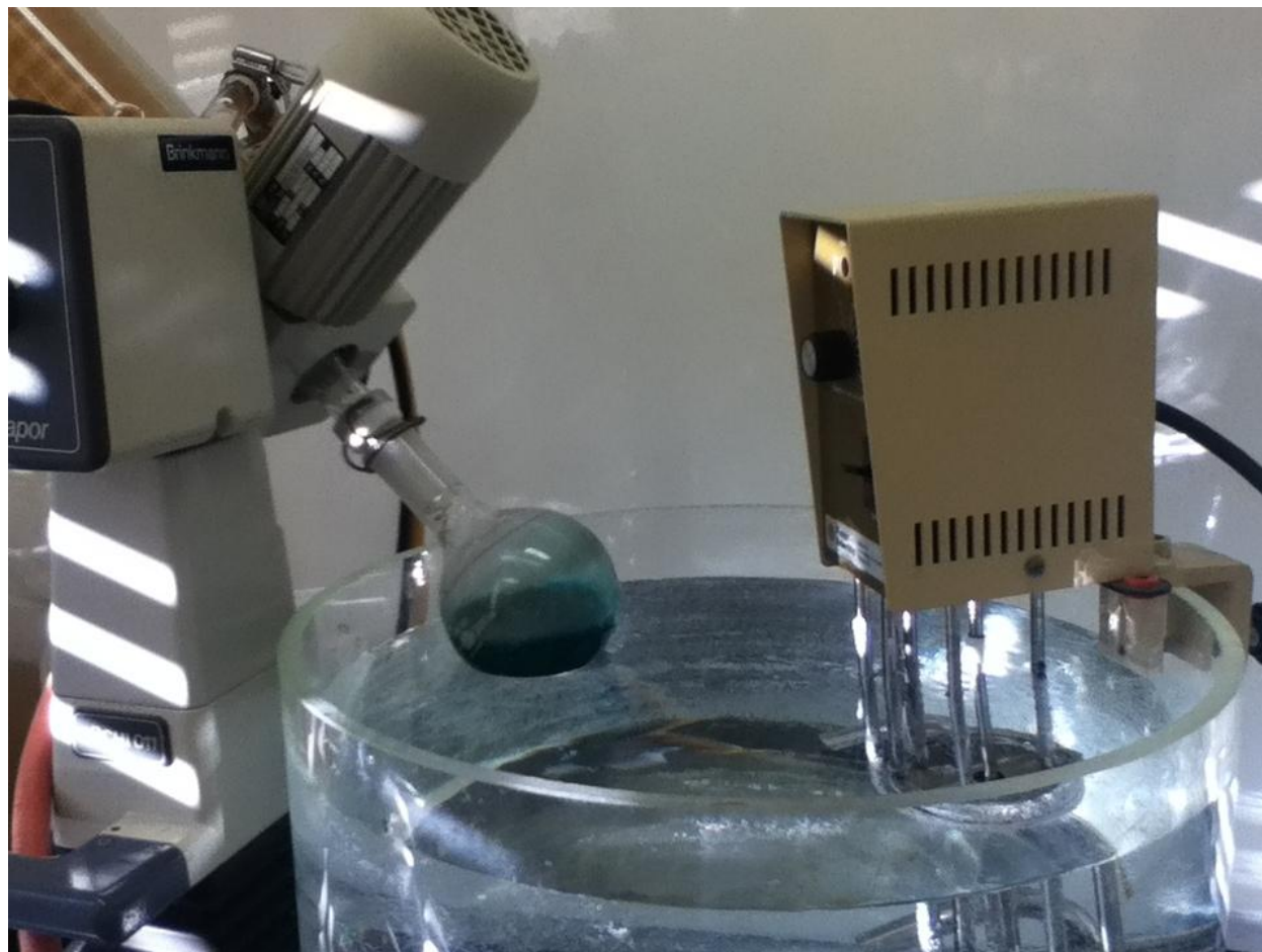
Figure 2.2: Rotary evaporation of chlorobenzene from reaction mixture
