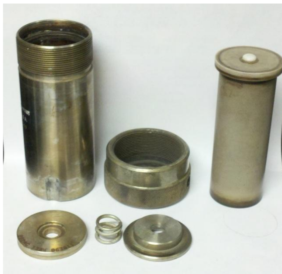
FIGURE 11 - Hydrothermal Autoclave with 50mL Teflon Vessel
