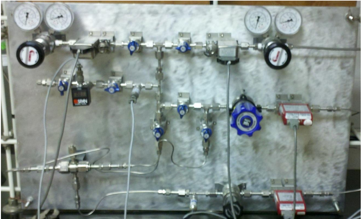
FIGURE 18 - Stainless Steel High Pressure Gas Separation System Model No: 4576A
