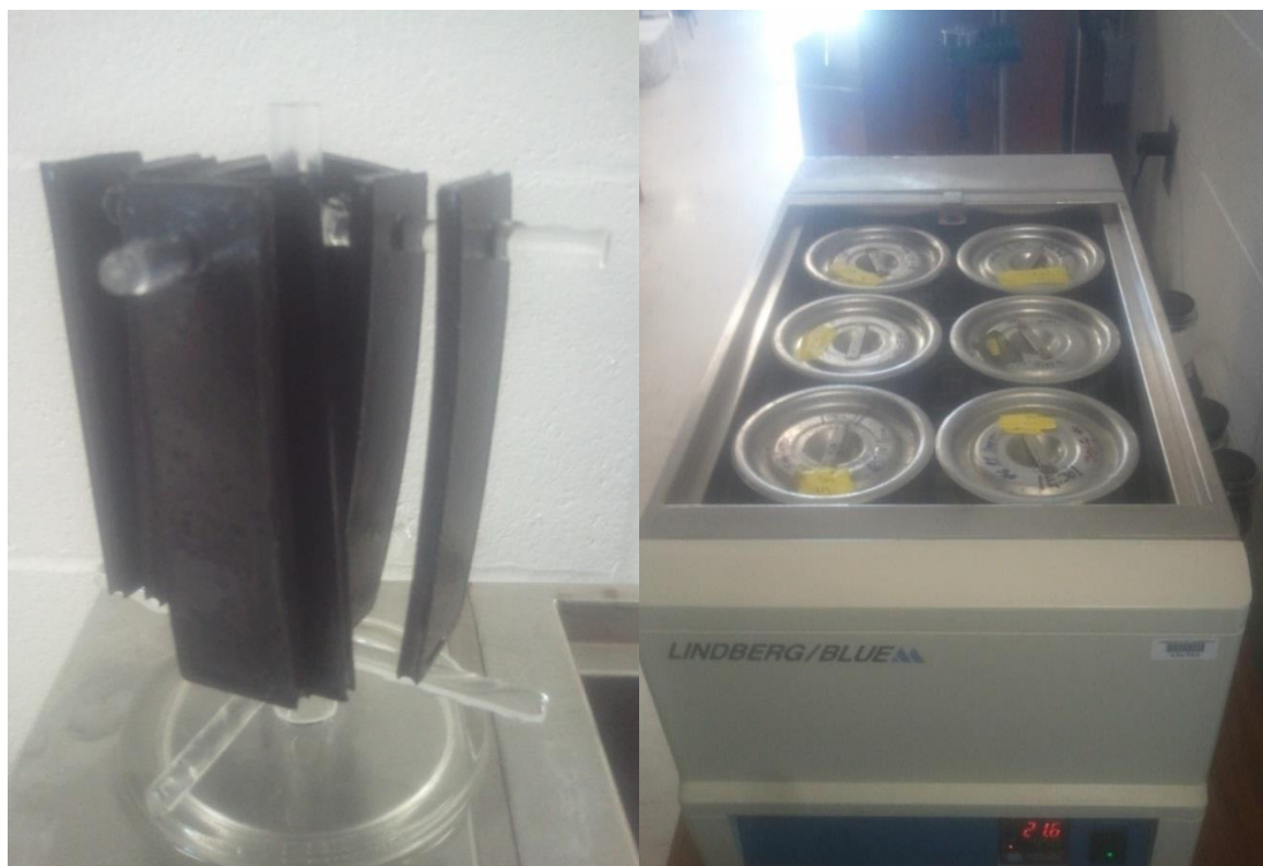
Figure 10. Rubber Samples on Glass Tree (left) and Sample Containers in Hot Water Bath (right)
