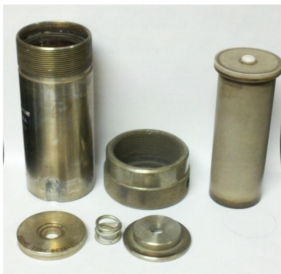
Figure 7 Hydrothermal Autoclave with 50mL Teflon Vessel 36
