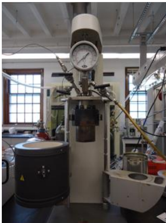
Figure 12 Parr Reactor Model 4576A
