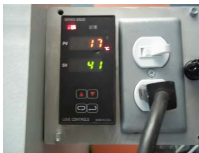
FIGURE 14: 8500 Series microprocessor based temperature control
