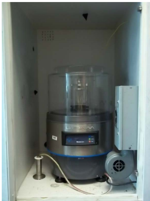
FIGURE 13: LAB-RAM Resonant Acoustic Mixer and centrifugal heater in heating box
