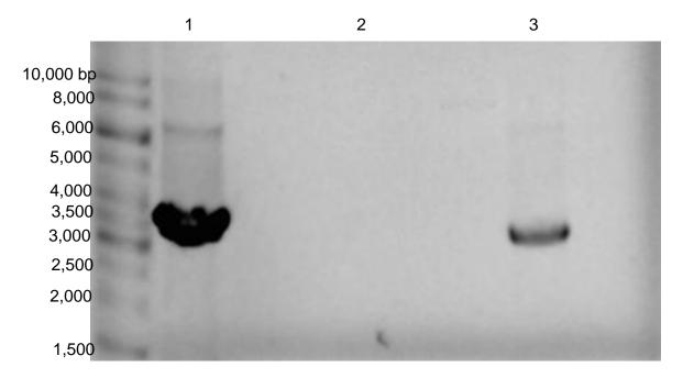
Figure 6: Analyzing the PCR Reaction Products of UvrA Gene. Products of PCR reaction using pSST10\_UvrA plasmid as the template as the positive control (Lane 1). Products of PCR reaction using dd-H<sub>2</sub>O as the template as the negative control (Lane 2). Purified PCR products were double-digested with restriction enzymes NdeI and XhoI (Lane 3).
