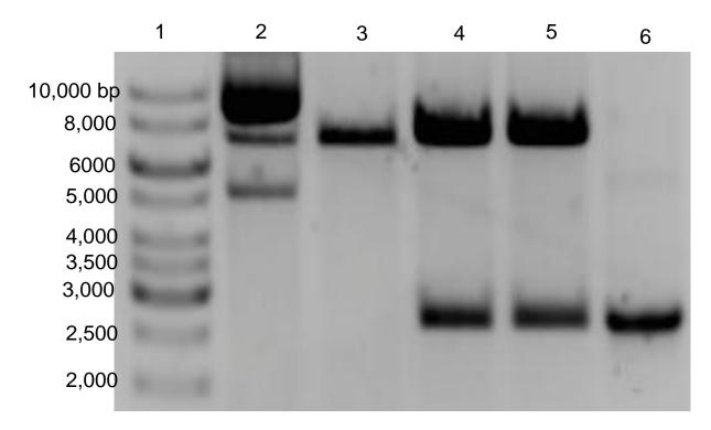
Figure 11: Confirmation of the amplified construct of pTYB2\_*Uvr*A with restriction enzymes Nde I & Xho I. DNA ladder (Lane 1). Circular vector pTYB2 plasmid (Lane 2). Double-digested vector pTYB2 with NdeI & XhoI (Lane 3). Double-digested plasmid (from colony B1) with Nde I & Xho I (Lane 4). Double-digested plasmid (from colony B2) with Nde I & Xho I (Lane 5). Protein *Uvr*A from pool-32B (Lane 6).
