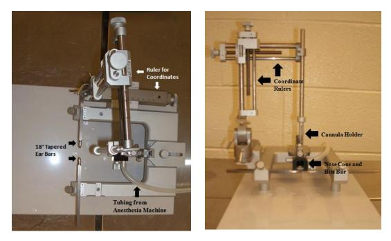
Figure 4: Two views of the stereotaxic apparatus depicting coordinate rulers, ear bars, tubing from anesthesia machine, nose cone, bite bar, and cannula holder.
