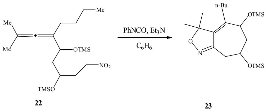
Scheme 5: Allene-intramolecular nitrile oxide cycloadditions in presence of bulky group
