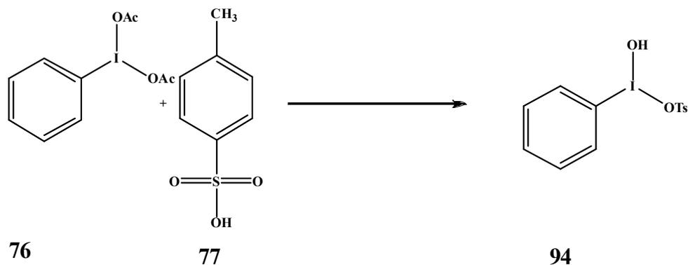
Scheme 25: First mechanistic step in the synthesis of tosyloxycyclohexanone (**78**)
