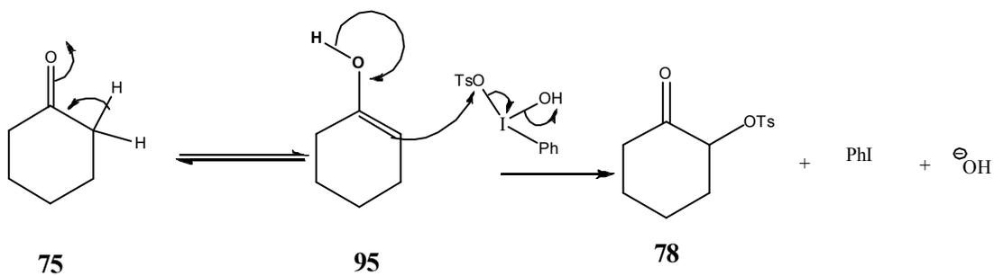
Scheme 26: Second mechanistic step in the synthesis of tosyloxycyclohexanone (**78**)
