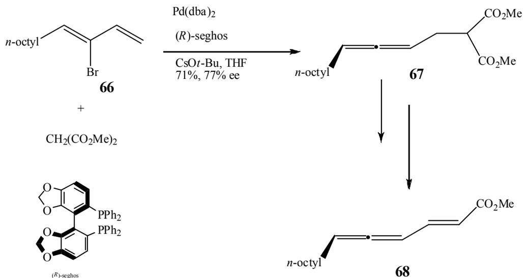
Scheme 18: Allene synthesis by Pd catalyzed  $\text{S}_{\text{N}}2'$  substitution of conjugated dienes
