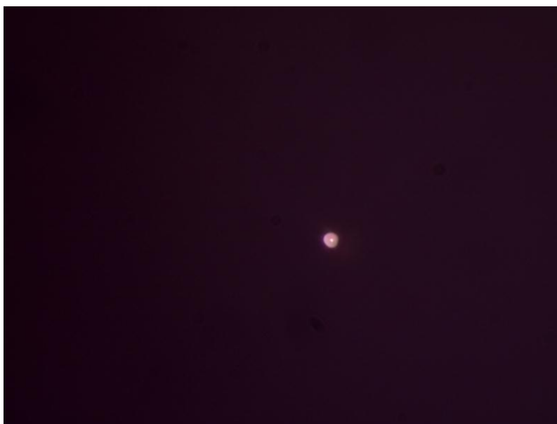
Figure 7: Top view of the optical microscopic image of a well-polished nanometer-sized Au electrode. The magnification is 1000x
