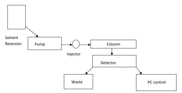
Figure 5: Schematic representation of high performance liquid chromatography
