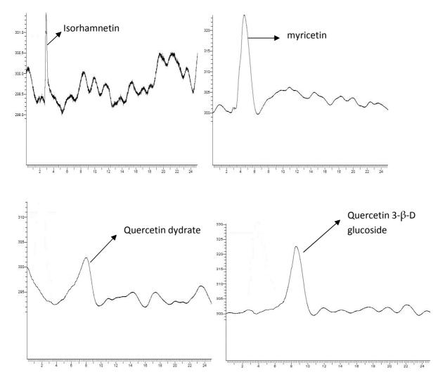
Figure 7: HPLC chromatograms of, isorhamnetin, myricetin, quercetin dydrate and quercetin-3- $\beta$ -D glucoside samples using 45:55 methanol:deionized water mobile phase. The retention times were identified for the standard compounds from the chromatograms.
