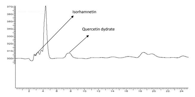
Figure 10: HPLC chromatogram of commercial organic red onion sample using 45:55 methanol: deionized water mobile phase. Quercitin dydrate and Isorhamnetin were the compounds that were observed in this sample when compared with the retention times of the standard compounds.
