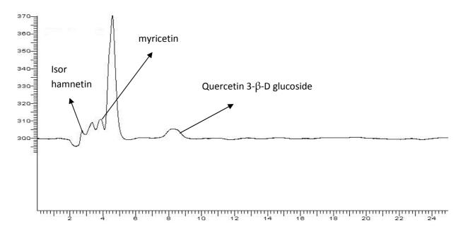
Figure 9: HPLC chromatogram of commercial organic white onion sample using 45:55 methanol: deionized water mobile phase. Quercitin 3- $\beta$ -D glucoside, isorhamnetin and myricetin were the compounds that were identified based on the retention times of the standard compounds.
