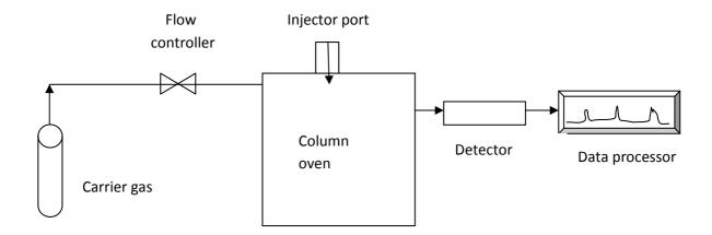
Figure 6: Schematic representation of gas chromatography
