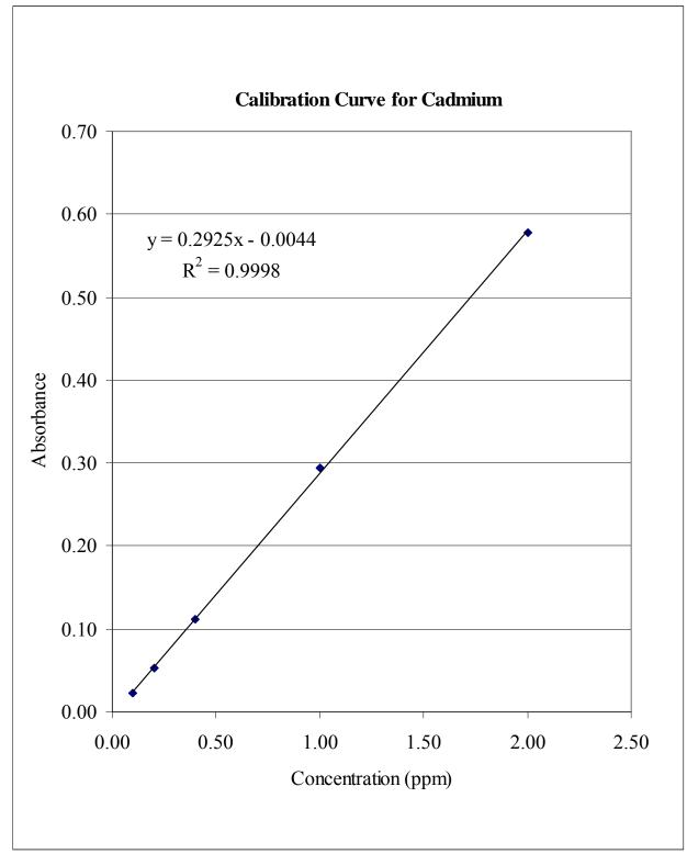
Figure 17. Calibration curve for cadmium.
