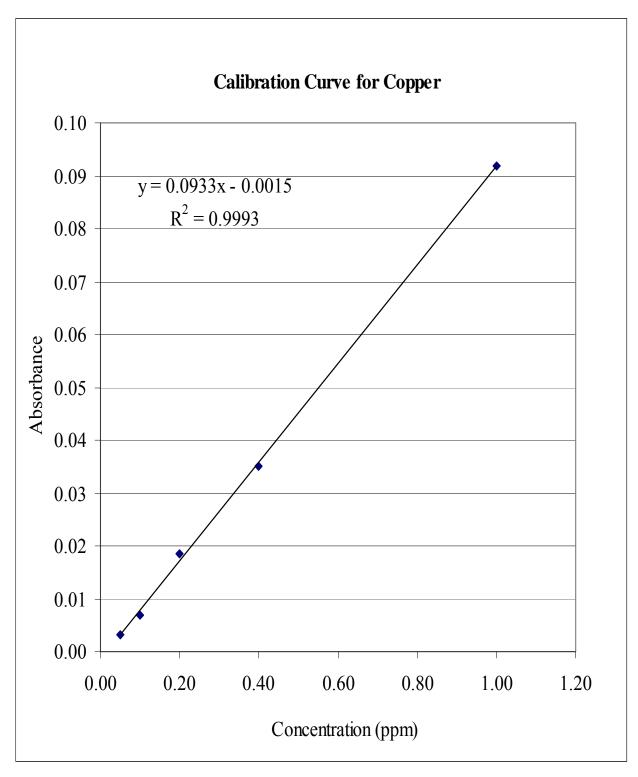
Figure 13. Calibration curve for copper
