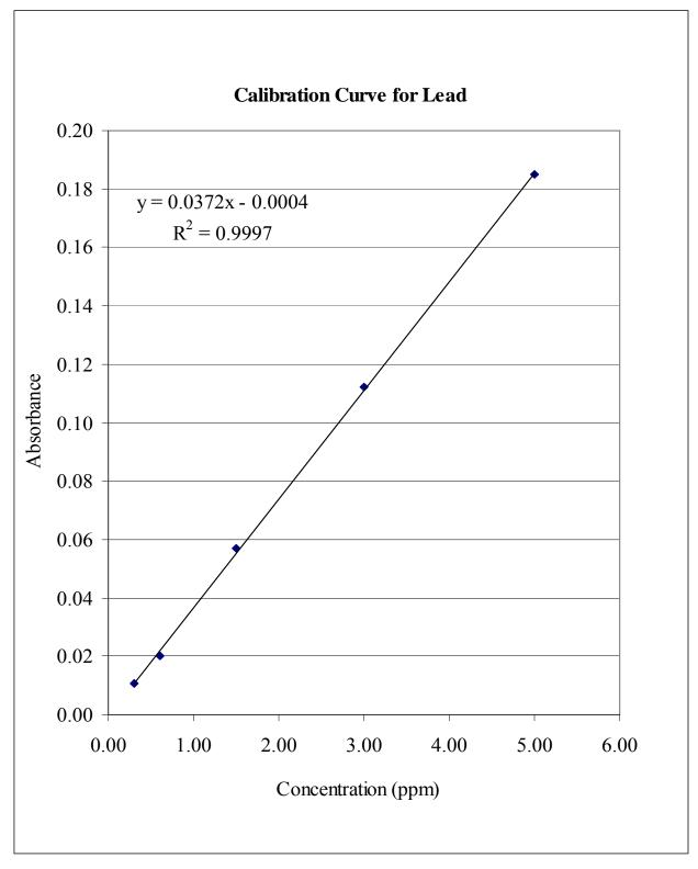
Figure 16. Calibration curve for lead.
