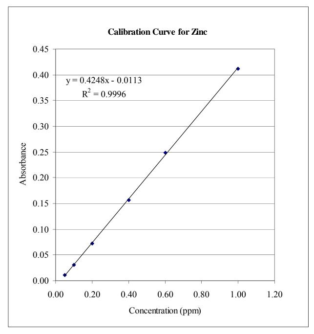
Figure 12. Calibration curve for zinc.
