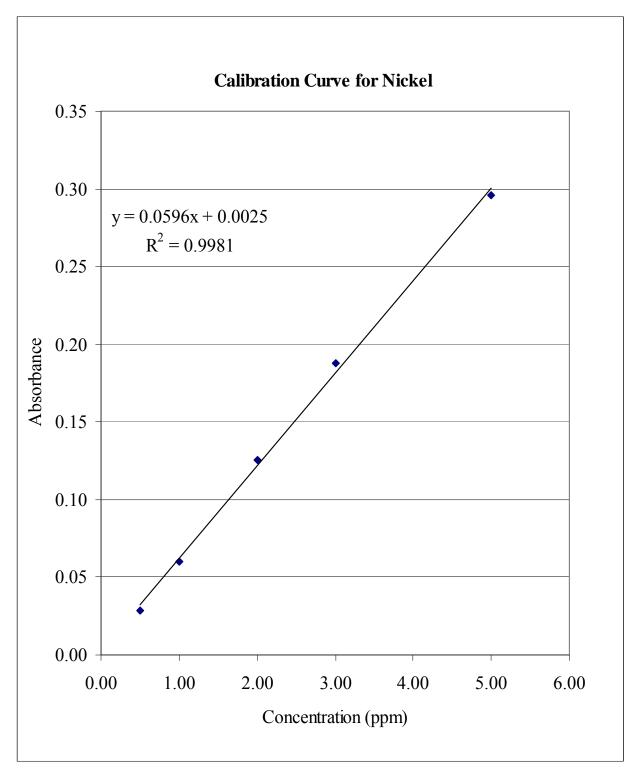
Figure 15. Calibration curve for nickel
