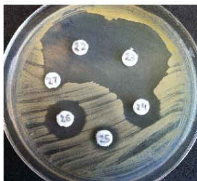
Figure 20: HPLC chromatogram for scale-up 2, run 3. Discs 16, 18, 19, and 20 corresponded to the first set of peaks, discs 22, 23, and 24 correspond to the large peak in the middle, and discs 25 and 26 correspond to the smaller last peak.
