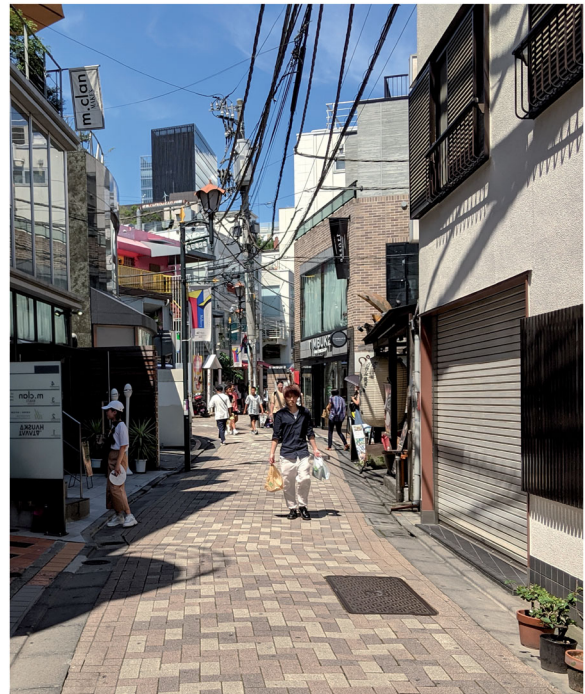
Figure 2. Shibuya City, Tokyo (Japan). The right-of-way is approximately 13 to 16 ft wide and provides a shared space for pedestrians and motor vehicles. Photo credit: Felix Vazquez.
