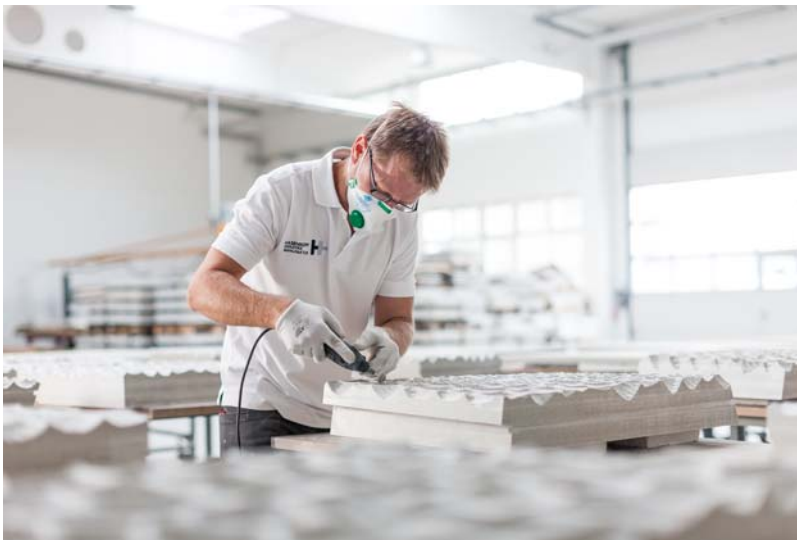
Figure 4. The processing of the innovative acoustic panels for the Elbe Philharmonic Hall, for which Hasenkopf Industrie Manufaktur GmbH was commissioned. © Christian Höhn | www.hasenkopf.de .
