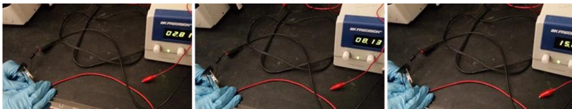
Figure 57: Bending of cellulosic plastic sample connected to a red LED and a DC Power Source at 2.81 V (left) 8.13 V (middle) and 15.0 V (right)
