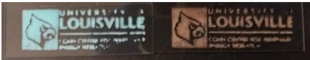
Figure 22: Example of visible change of a \text{Cu}_2\text{NO}_3(\text{OH})_3 sample before (left) and after (right) IPL
