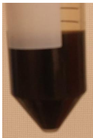
Figure 19: Photograph of 20 mg/mL GO solution displaying great ink stability nearly five months after it was formulated
