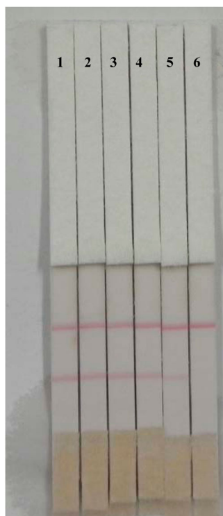
Figure 6. Analysis of cyproheptadine concentration with strip in pig urine (1 = 0 ng/mL, 2 = 0.25 ng/mL, 3 = 0.5 ng/mL, 4 = 1 ng/mL, 5 = 2.5ppb, 6 = 5ppb, the strip cut-off completely at 5 ng/mL of cyproheptadine).
