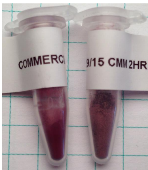
Figure 4.1 Commercial \text{Ce}_2\text{S}_3 (left) compared to solvothermally prepared cerium sulfide powder (right).
