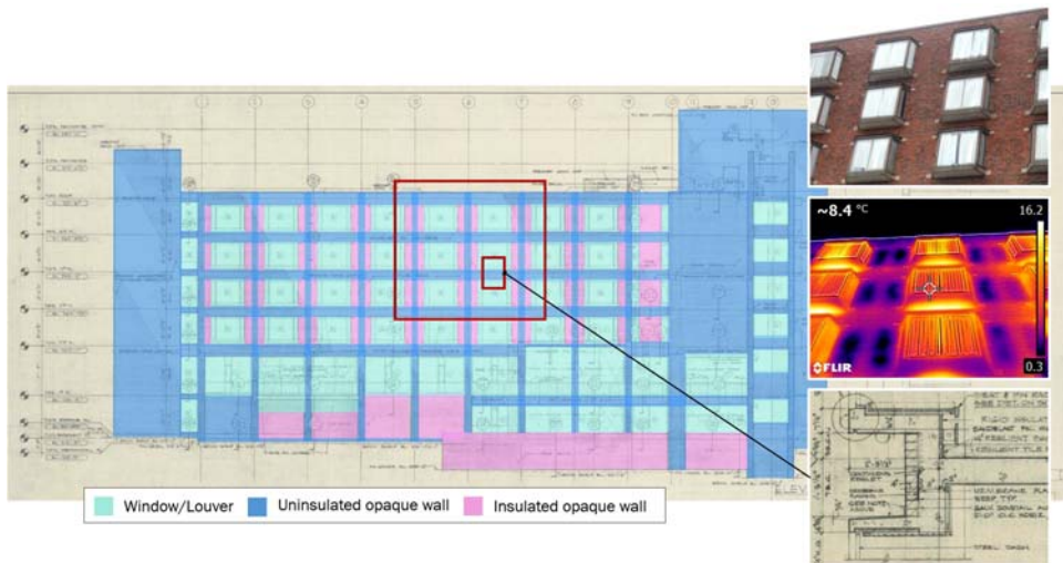
Figure 11. Axonometric rendering and thermal model results of existing bay windows of MacGregor Hall.
