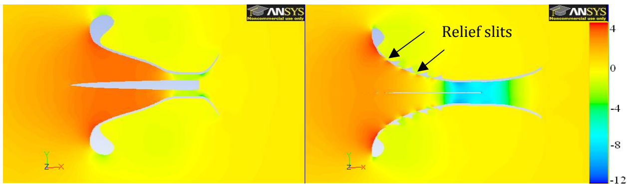
Figure 35: Comparison of gauge pressure within concentrator before (left) and after addition of relief slits. (Pa)
