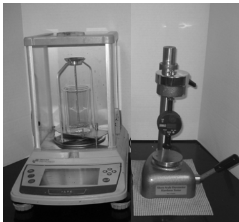
Figure 2.6 Analytical balance with water submersion aperture (left) and digital durometer (right)
