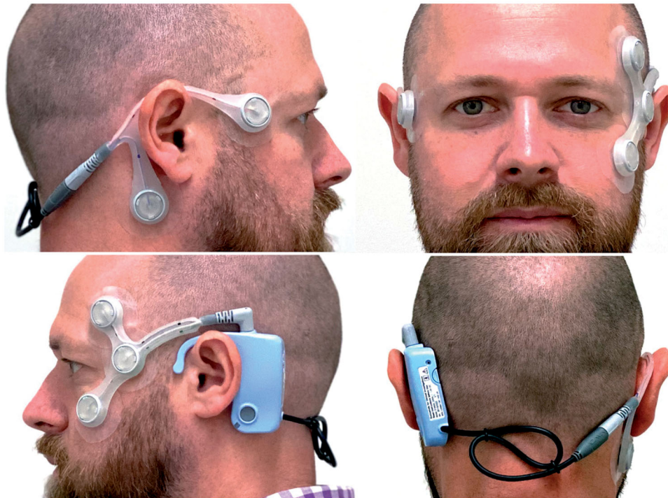
Figure 1. The appearance of the CAVA ® device when worn on the head. The device includes a reusable logging module and two, single-use electrode mounts. Five ECG electrodes are placed at specific sites on the face to record the corneo-retinal potential produced by the eyes. A button on the logging unit allows the patient to activate the device's event marker, which causes the device to log the date and time of the button press. The button can also be used to initiate a status check of the device, the results of which are confirmed visually by the device's status LED. The status checking feature provides feedback regarding battery level, the connection of the device's electrodes, and confirmation of event marker activation.
