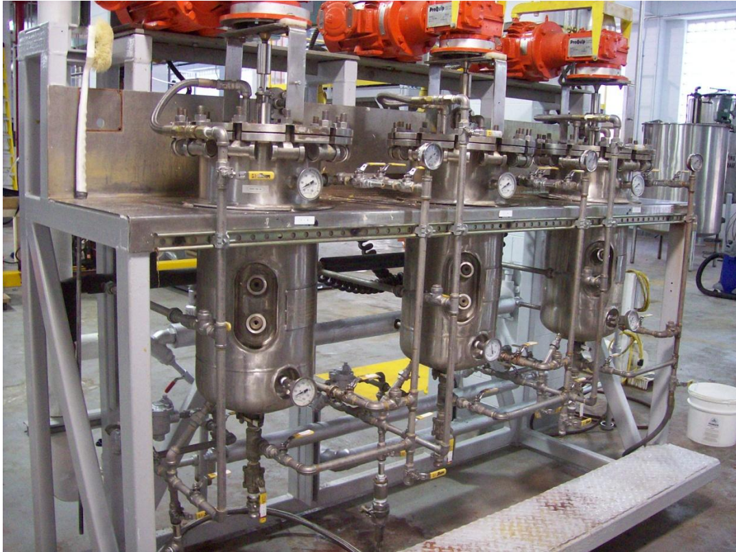
FIGURE 1 – Mashing Cookers. Mashers are cooked in 40 L steam-jacketed cookers.
