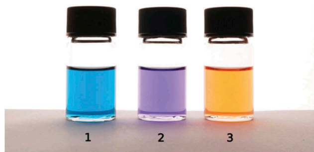
Figure 2. (Colour online) Photograph of solutions of the dyes at ca. 1 \times 10^{-4} \text{ mol dm}^{-3} in dichloromethane.
