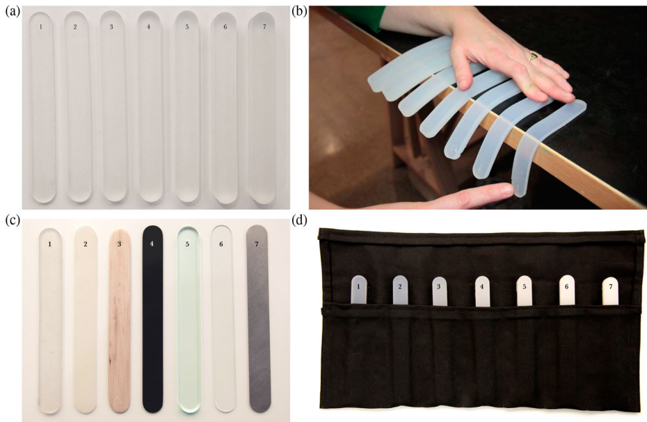
Figure 4. (a,b) A stiffness/flexibility material-object set made from one material (silicone rubber) of varying thickness in 2 mm increments to illustrate that Young's Modulus remains constant whilst stiffness varies considerably as a result of the form of the object; (c) The seven multi-material samples exploring stiffness were made from a selection of materials with different Young's Modulus: two different grades of silicone rubber, balsa wood, polystyrene, acrylic, glass and stainless steel. (d) An opacity/transparency material-object set made from one material (silicone rubber) with the same shore hardness, shape and dimensions but different quantities of white dye in a measured gradation.
