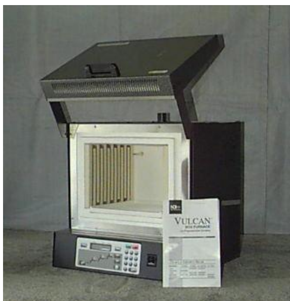
FIGURE 8 - Ney® Vulcan 3-550 Furnace Dentsupply Ceramco International Serial No.: 9493308 York, PA 17404 24
