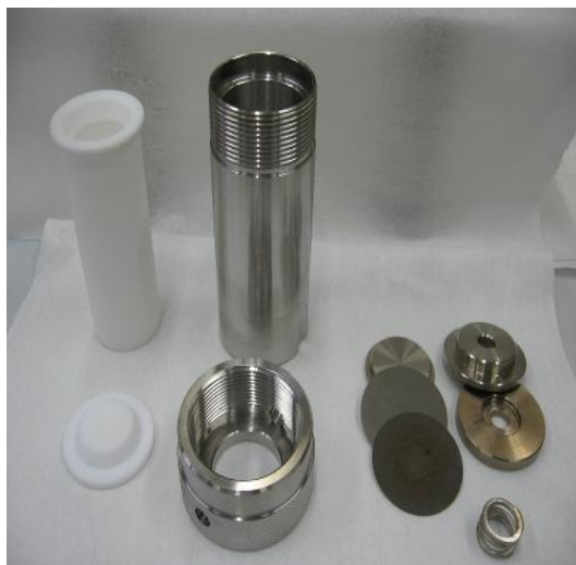
FIGURE 7 - Hydrothermal Autoclave with 50mL Teflon Vessel 23
