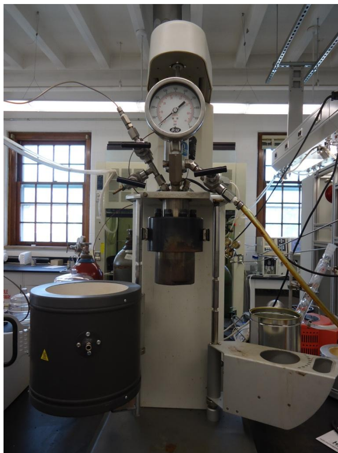
FIGURE 14 - Stainless Steel High Pressure Parr Reactor Model No: 4576A
