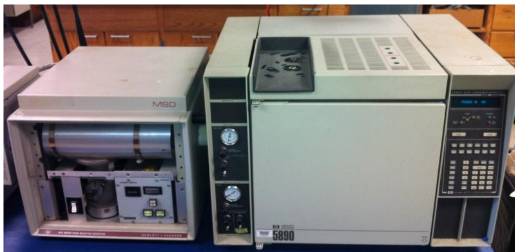
FIGURE 15 - GC-MS HP 5890 Gas Chromatograph equipped with 5970 Mass Selective Detector
