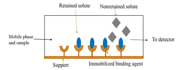
sufficient mechanical stability and efficiency that is needed for use in the high pressure in HPLC, the support must be selected and optimized acordingly [3,5]. The use of an HPLC- type of support, results in a method known as high-performance affinity chromatography (HPAC), which has better precision and a much faster speed than are usually present in traditional affinity chromatography [3,5]. Automation with the use of HPLC systems also is relatively easy to accomplish in HPAC [1,4,5].
