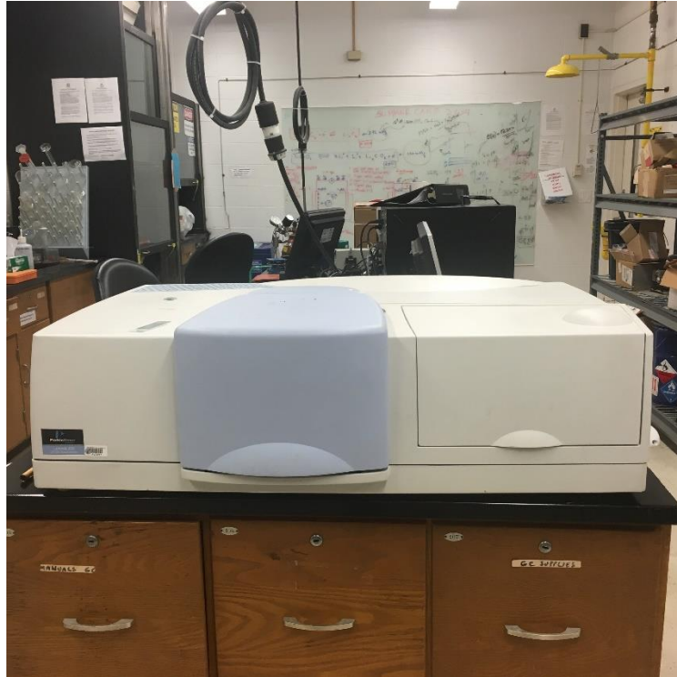
FIGURE 5 - UV Vis Spectrometer used for polymer detection (Lambda 950 model)
