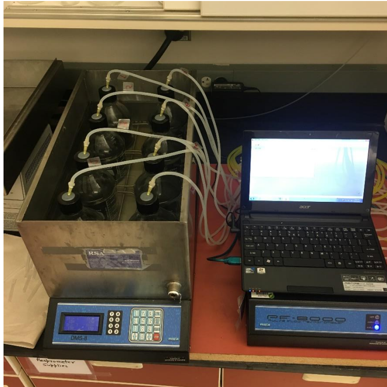
FIGURE 4 - Lab scale respirometer for anaerobic digestion (PF-8000 model)
