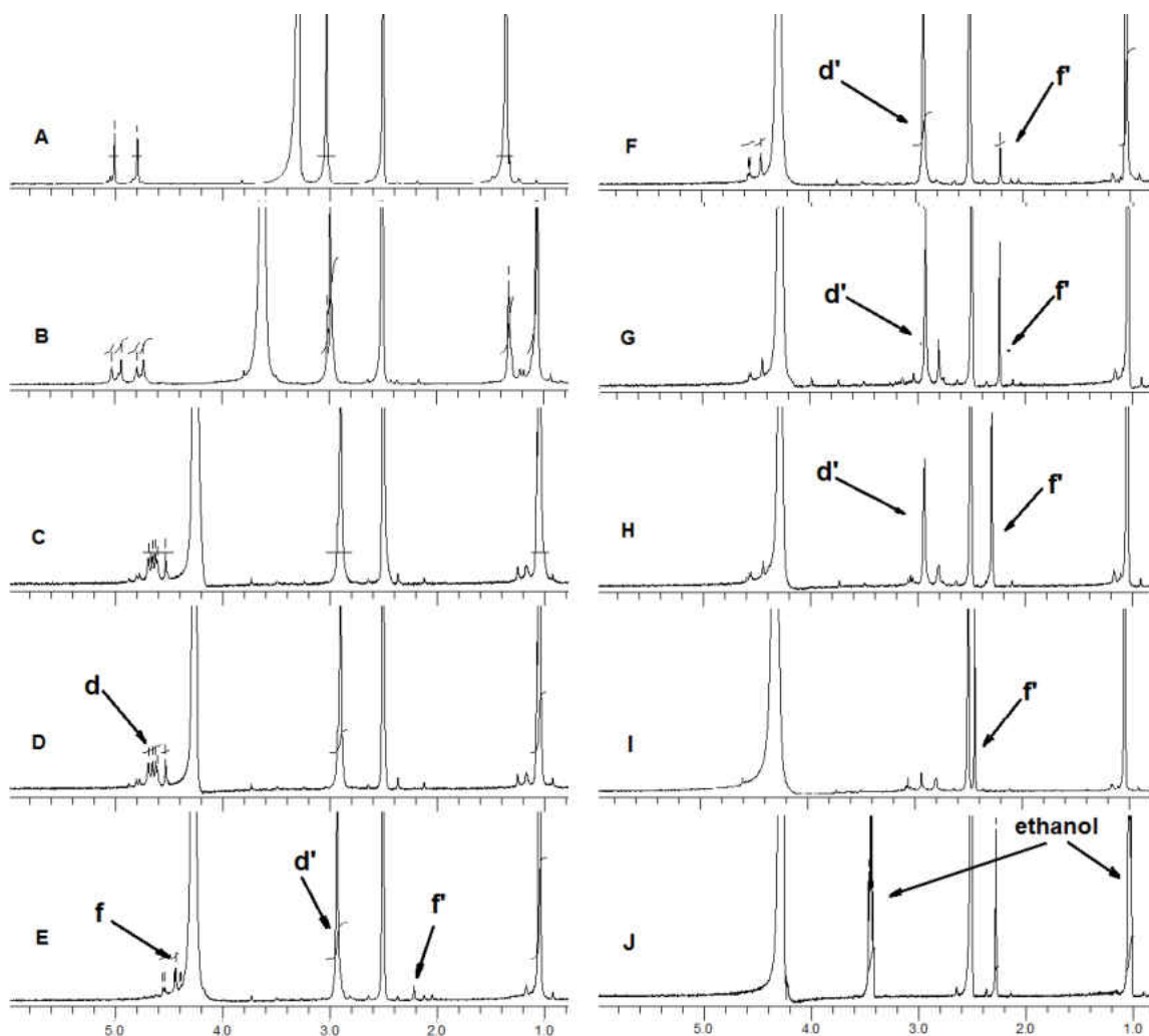
Figure 2-17. ^1\text{H} NMR analysis of 4c in deuterated DMSO, \text{D}_2\text{O} , and \text{H}_2\text{O}_2 : (A) ^1\text{H} NMR of 4c (0.003 mmol) in DMSO only; (B) 30 min in mixture of DMSO (300 \mu\text{L} ), \text{D}_2\text{O} (20 \mu\text{L} ), and pH8 buffer (10 \mu\text{L} ); (C) additional 30 min after added additional DMSO (60 \mu\text{L} ) and \text{D}_2\text{O} (210 \mu\text{L} ) in B; (D) additional 3 h after added additional DMSO (60 \mu\text{L} ) and \text{D}_2\text{O} (210 \mu\text{L} ) in C; (E) 3 min after addition of \text{H}_2\text{O}_2 (3 equiv.) in D; (F) 30 min after addition of \text{H}_2\text{O}_2 ; (G) 3 h after addition of \text{H}_2\text{O}_2 ; (H) 18 h after addition of \text{H}_2\text{O}_2 ; (I) 50 h after addition of \text{H}_2\text{O}_2 ; (J) Trimethyl amine ( \text{NMe}_3 ) in ethanol with addition of 1 M HCl (10 \mu\text{L} ).
