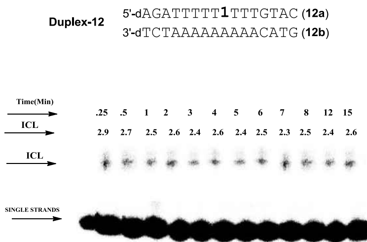
Figure 32. PAGE analysis of photolytic cleavage of ICL from duplex-12
