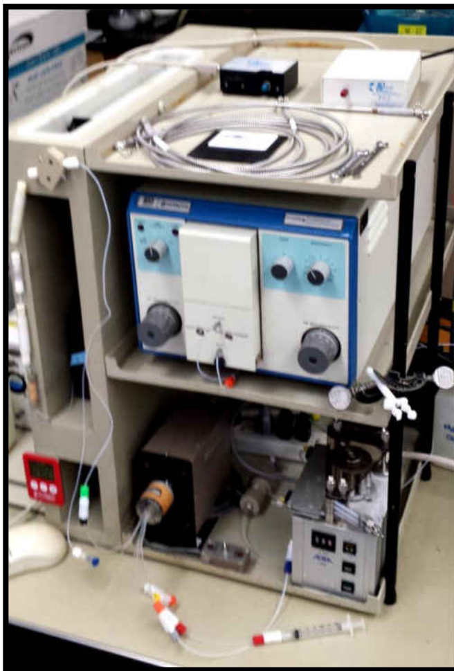
Figure 2-9. Photograph of the RP-LC system.
