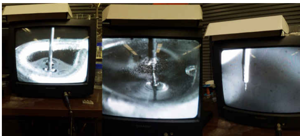
FIGURE 3.7: Three stages of the tip etching process, the first shows early stages of etching, in the second, clear etching of the tungsten wire can be observed, and finally after the lower wire has fallen.
