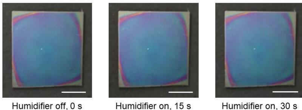
Figure 3.17. Photographs (top view) of the thin film of PC deposited on iridium-coated glass substrate in response to mist created by a humidifier. Thickness of the iridium film is 5 nm. Scale bar: 1 cm.
