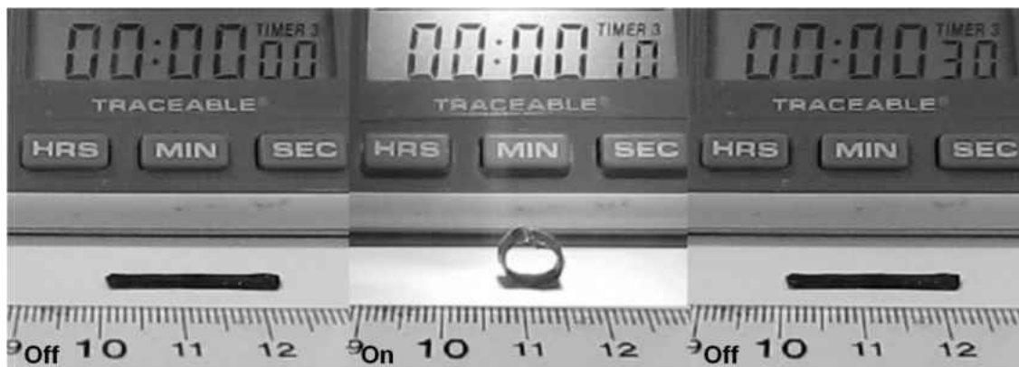
Figure 16. Photo images of a 0.1 wt% SWNT-LCE/silicone bilayer film as it responds to IR irradiation.
