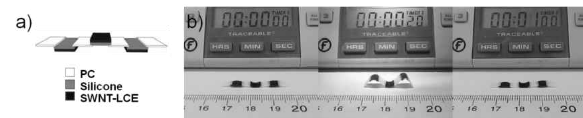
Figure 20. a) Schematic illustration of the foldable structure. b) Folding and unfolding of the foldable structure as IR source is turned on and off.
