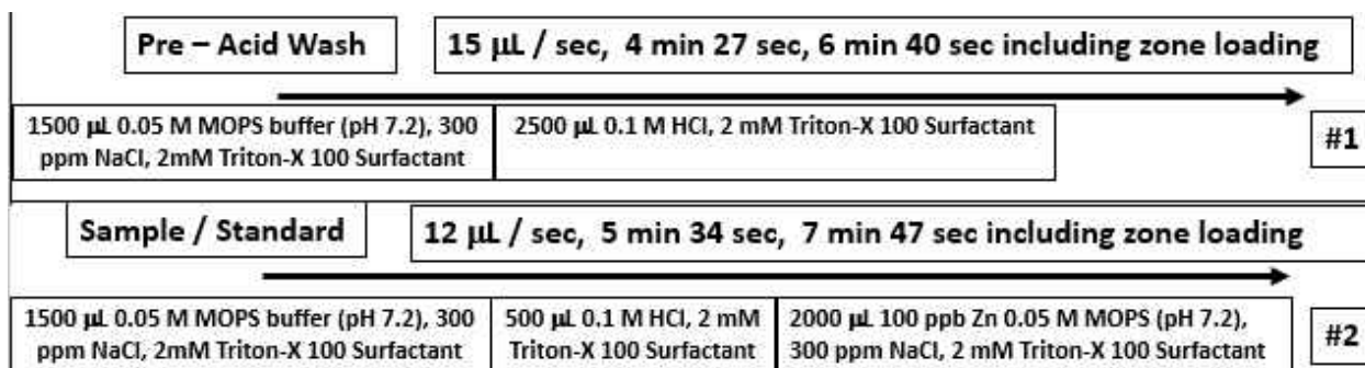
Figure 11. Experimental design. Analysis would alternate between Pre – Acid Wash and Sample / Standard runs to ensure removal of previous run’s metal from dye film.
