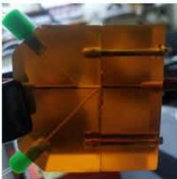
Figure 10. Photograph of the flow cell used in SIA, showing the optical path as well as the 'Z'-type flow path. 50
