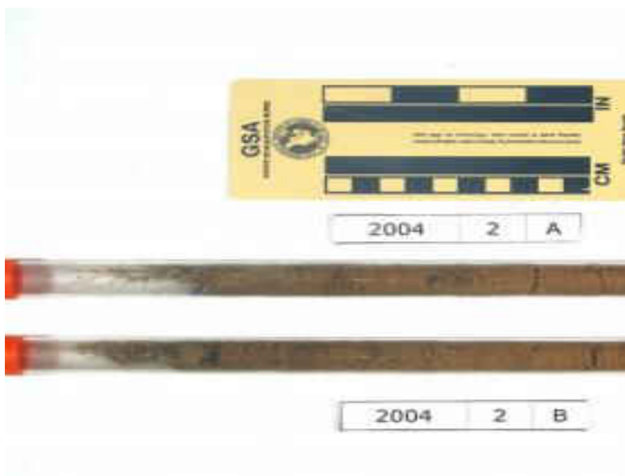
Figure 17. Photograph of a typical soil core sample. The top of the core is orange-capped. Photograph by T. Grundl, September 2007.
