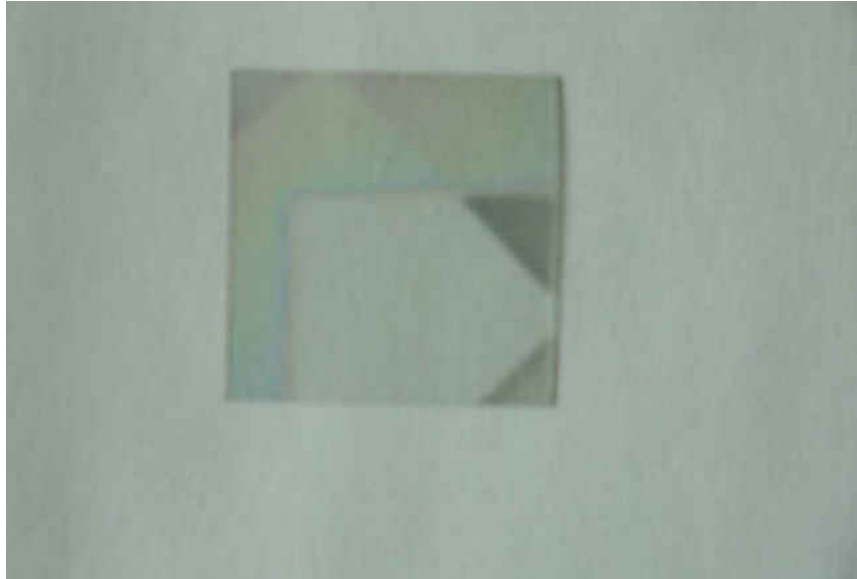
Figure 4.18. Sputter coating of \text{HfO}_2 with the pattern seen on coverslip (analysis done by help of Elizabeth Hoppe).
