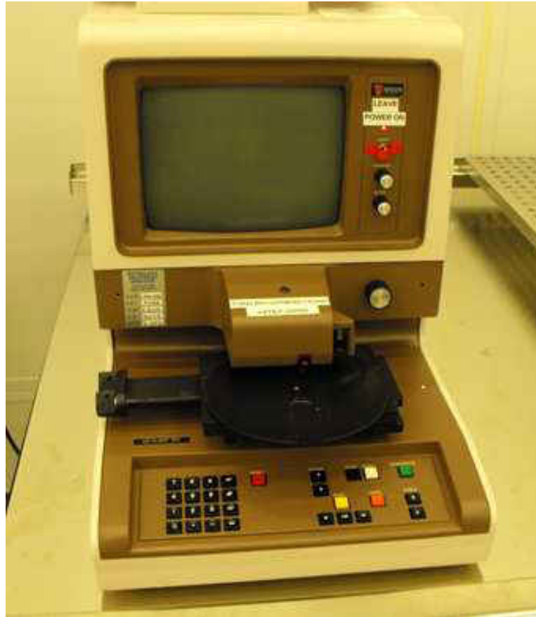
Figure 4.1. Thin film thickness measurement Tencor Alpha-Step 200 profilometer.
