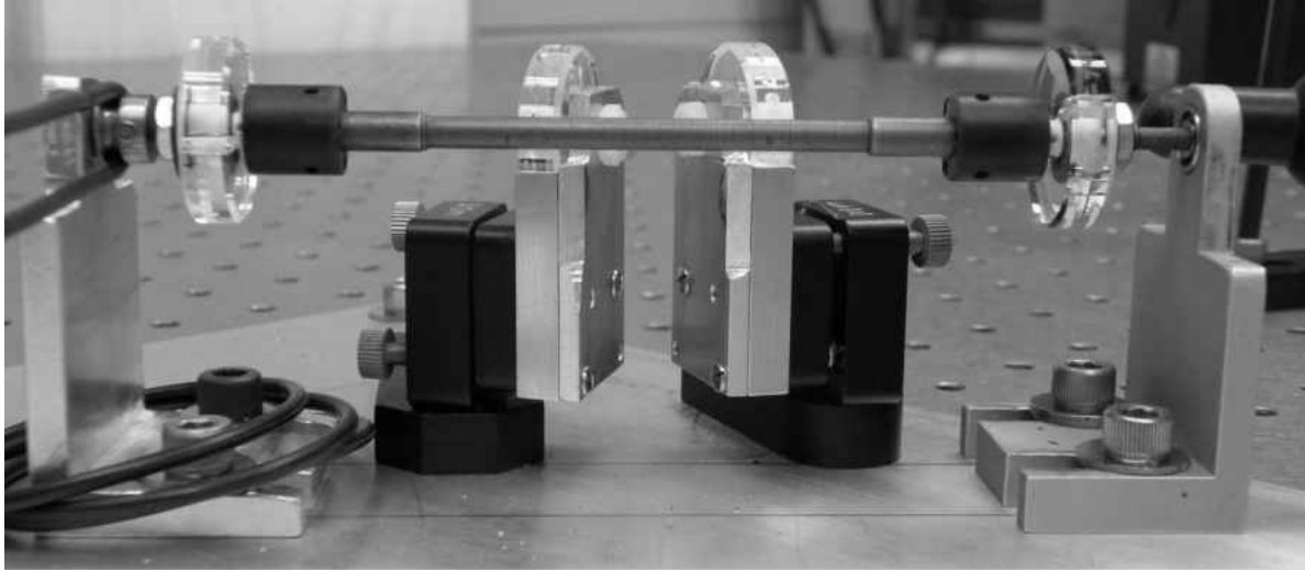
Figure 2-9 The P2 axle mount assemble. The unsupported axle, the weak “L-shaped” axle mounts, and the drive band not being separated from the mirrors lead to observable vibrations. Image taken from Reference 1.
