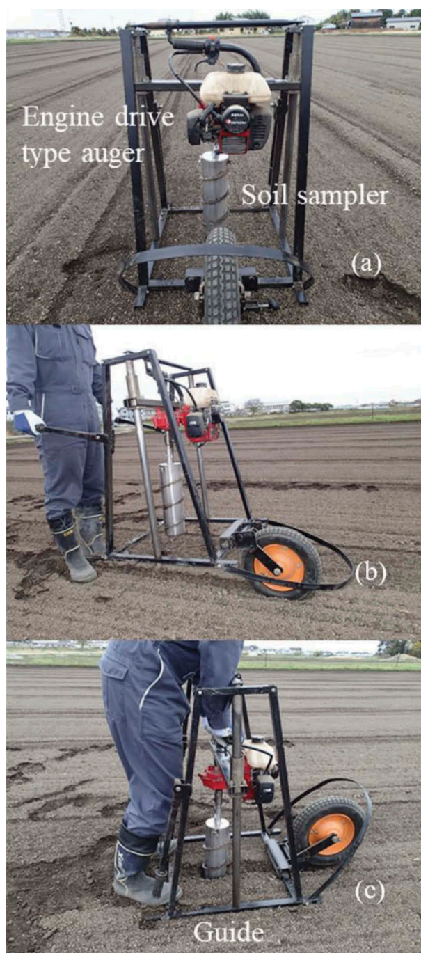
Figure 3. Soil sampler modified and used in this study (a). Hand-made carrier used to move sampler inside the field (b). A soil sample perpendicular to the ground could be collected by pushing soil sampler along a guide into the soil (c).
