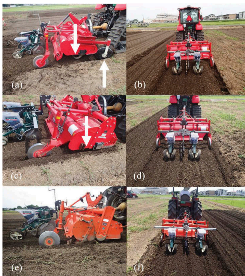
Figure 1. Sowing with one-operation shallow tillage with up-cut rotary tiller and side-disk (up-cut shallow tillage: UST) (a, b), one-operation conventional tillage with up-cut rotary tiller (up-cut conventional tillage: UCT) (c, d) and two-operation conventional tillage with down-cut rotary tiller (down-cut conventional tillage: DCT) (e, f). Pictures are from the side of (a, c, e) and behind (b, d, f) rotaries. The upward arrow in Figure 1(a) indicates side-disk attached to up-cut rotary tiller. Downward arrows in Figure 1(a,c) indicate the difference in the space between the side-board and the soil surface in UST and UCT.
