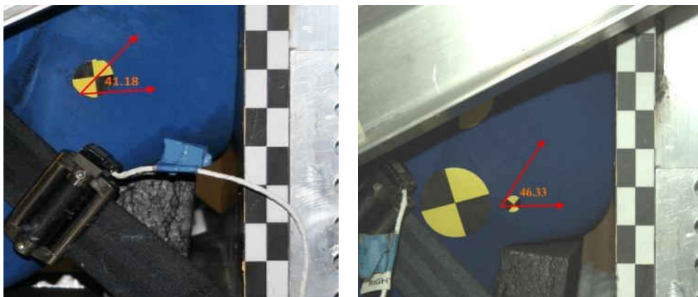
Figure 0-9: Pelvis angle measured by the Romer arm for Tests 3 and 4, respectively.
