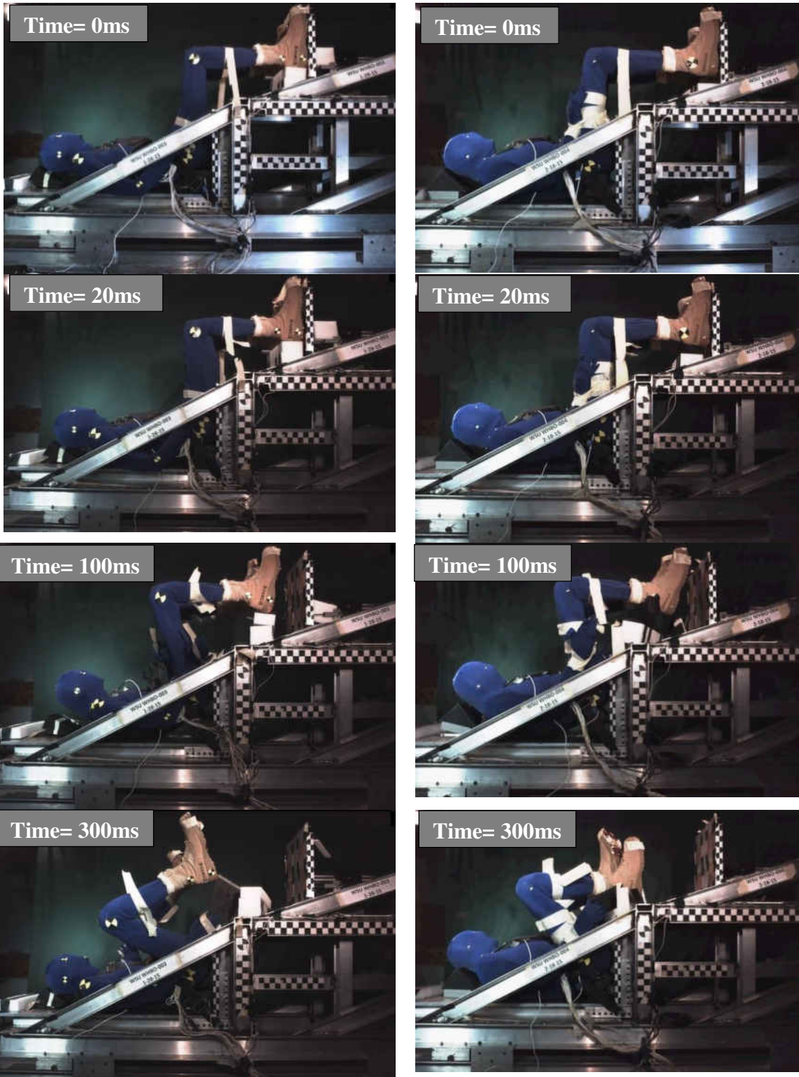
Figure 2-36: Kinematic comparison between WSU-003 and WSU-004 at different time points which includes: Time zero, 20, 100, 300 ms, respectively.
