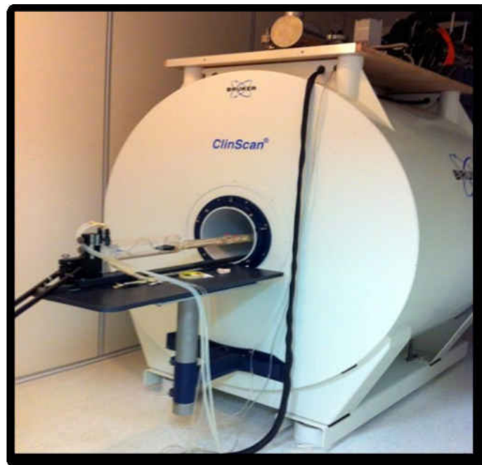
Figure 4-4: An image of the 7T MRI scanner from which the MRI data in this study was acquired.
