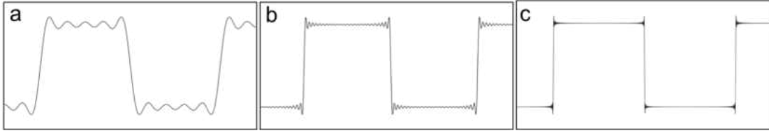
Figure 2.11, The effect of increasing the number of harmonics in approximating a square wave function. (a) 5 harmonics, (b) 25 harmonics and (c) 125 harmonics. It can be seen that the peak-to-peak difference of the overshoot and undershoot does not change. But they move closer to the discontinuity by increasing the number of harmonics. Image taken from Wikipedia.
