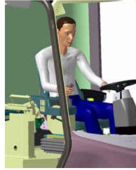
Figure 10: Posture analysis and vision study simulation with RAMSIS (Human Solutions, 2010b).
