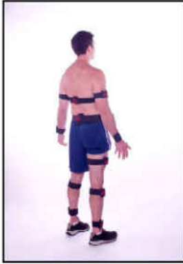
Figure 15: Image of FAB wireless sensor placement on the body (Biosyn, 2007).
