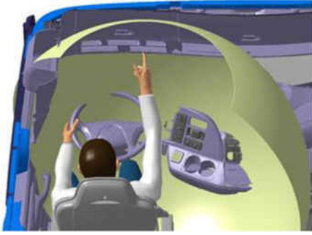
Figure 9: Posture analysis and reach study simulation with RAMSIS (Human Solutions, 2010b).
