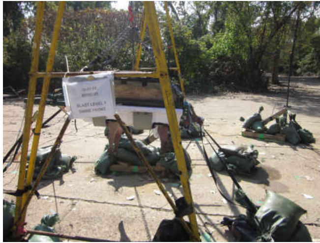
Figure 2.1: Instrumented swine test: the pig head was front to the blast wave
