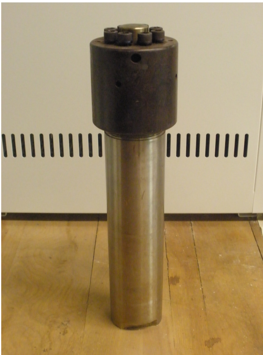
Figure 2.1. High pressure reactor used to hydrothermally convert cuttlefish bone ( \text{CaCO}_3 ) to hydroxyapatite. It has an outer diameter of 65 mm, an inner diameter of 39 mm, a height of 36 cm, and a volume of approximately 310 \text{ cm}^3 .
