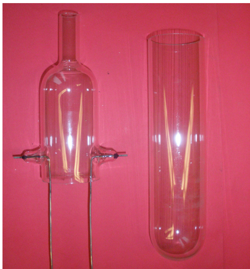
Figure 3.3. Sketch (top) and image (bottom) of the CVDP reactor.
