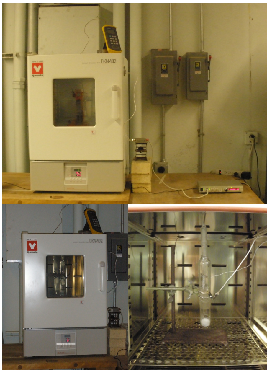
Figure 3.5. Images of the complete reaction setup (top), the convection oven with the CVDP reactor inside (bottom left) and the CVDP reactor inside the oven (bottom right).
