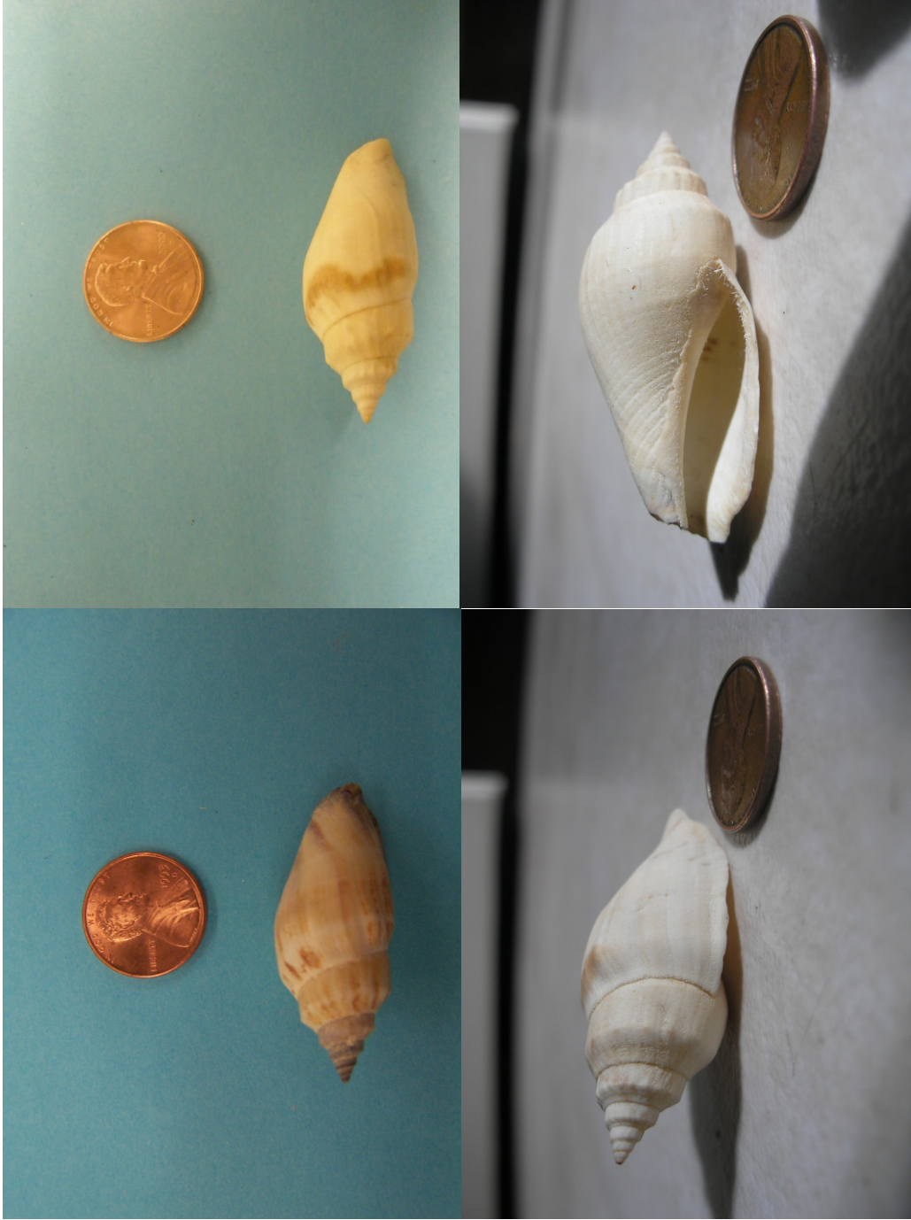
Figure 2.30. Images of (upper left) the shell of a young Strombus urceus in its original state and (upper right, bottom) the same shell after being converted to hydroxyapatite and reconstituted with PLLA via CVDP.
