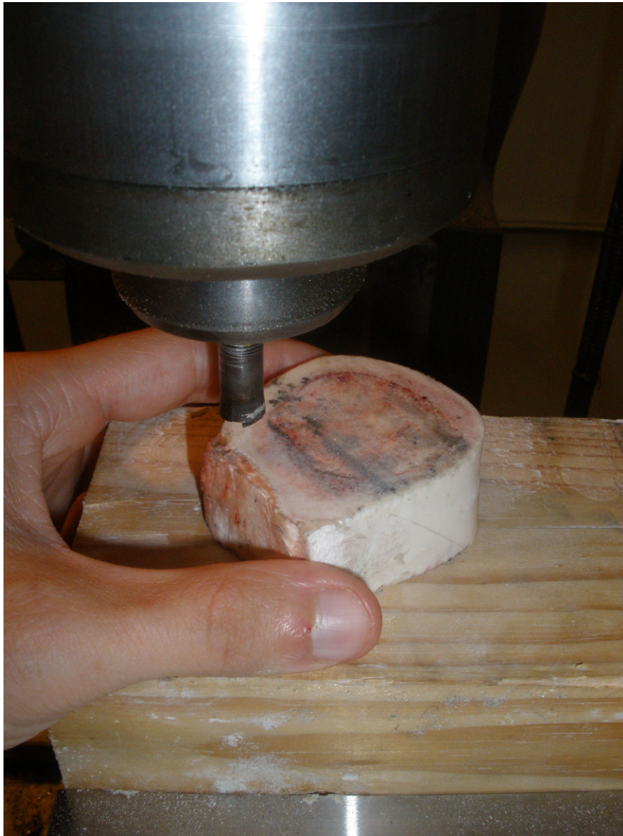
Figure 4.1. Cylindrical cortical bone plugs cut using an end mill and 6 mm dowel tool.
