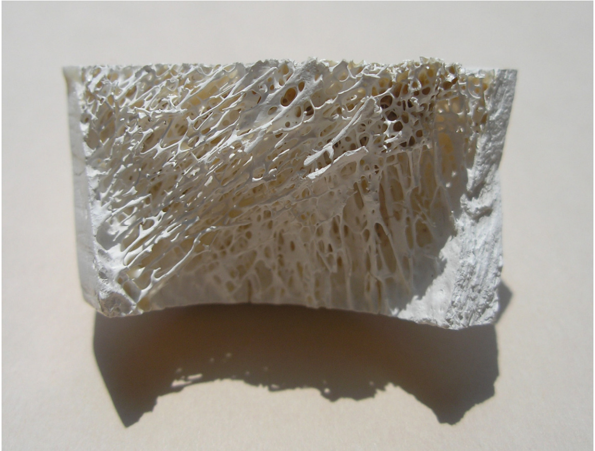
Figure 4.4. DBMS created from a diaphyseal section of bovine femur that was converted to anorganic bone, reconstituted with poly- \epsilon -caprolactone, and had the HA removed via extraction in 0.6 M HCl.
