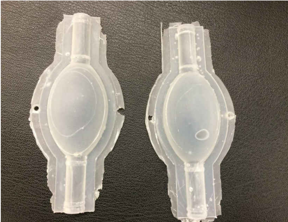
Figure 17: The two inner surface moulds made out of LSR
