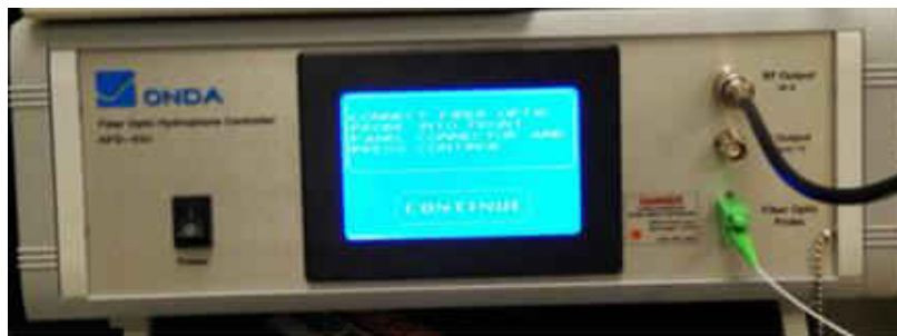
Figure 15. ONDA HFO-690 fiber optic hydrophone (pressure sensor).
