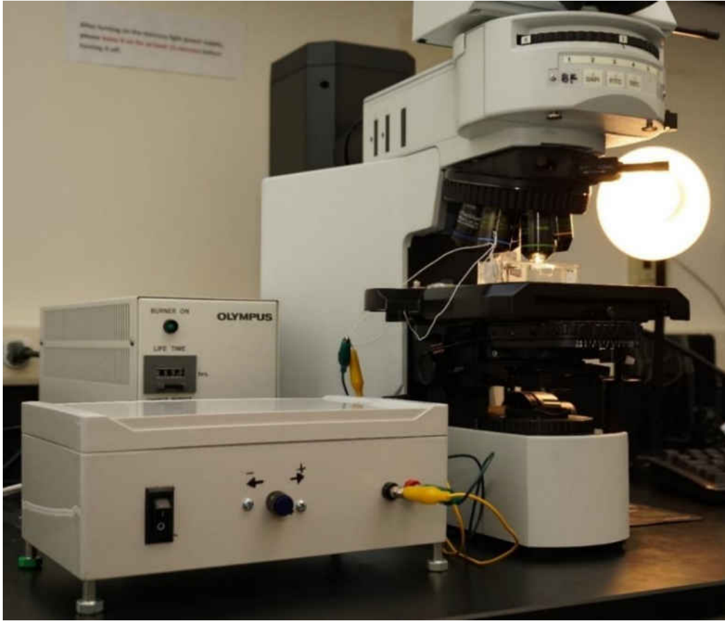
Figure 33. The whole setup of the bubble generator, which includes the driver, the chamber, and the microscope.
