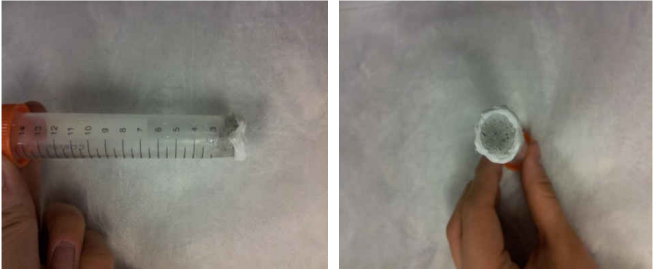
Figure 11 The gravity flow rate test. The scaffold was tightly sealed with the tube by silicon glue.
