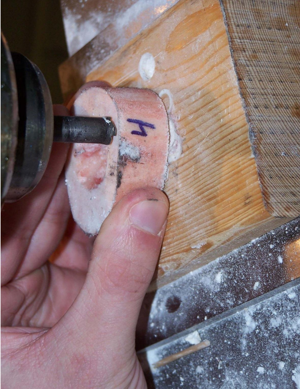
Figure 3.5. Image of a standard 6mm diameter bovine bone plug being cut from a section of bovine femur
