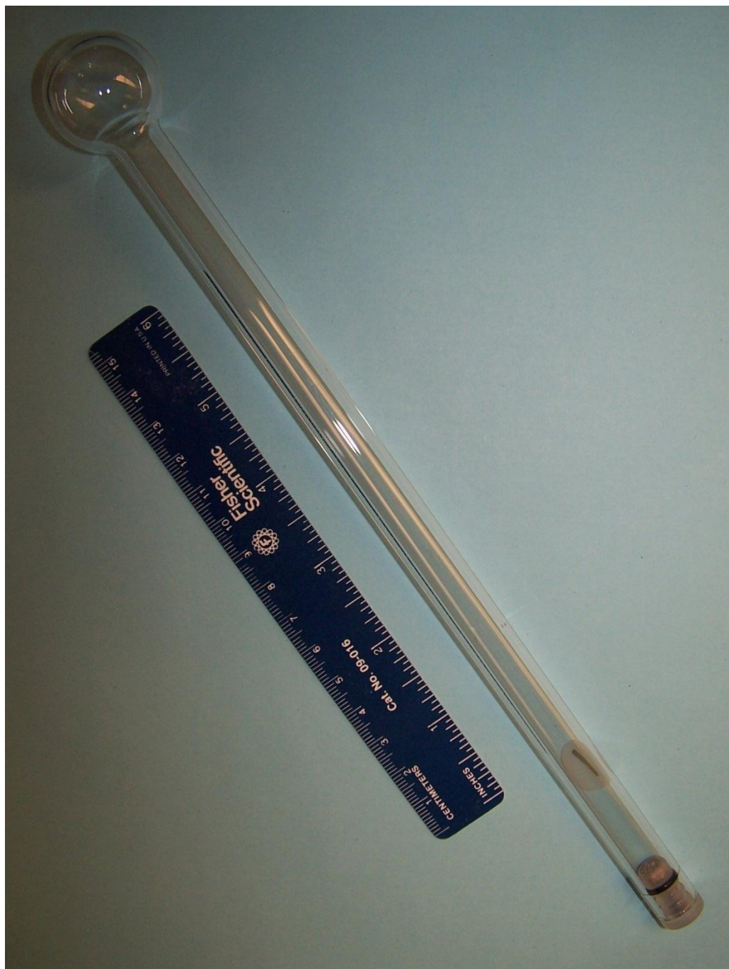
Figure 3.3. Typical surface area setup tube used in the Micromeritics® ASAP 2020
