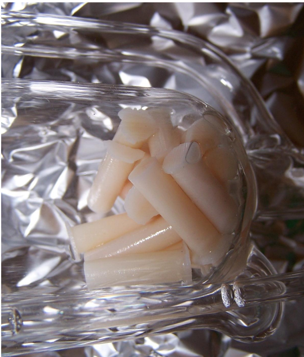
Figure 6.4. Extraction of bovine bone plugs used in the manufacture of compression and torsional test devices
