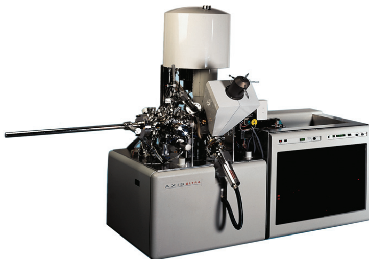
Figure 2.13: Kratos Axis Ultra DLD XPS instrument equipped with a hemispherical analyzer, dual Mg/Al x-ray anode, monochromatic Al x-ray anode and ion gun for sputter cleaning. The base pressure is typically less than 5 \times 10^{-10} Torr [21].
